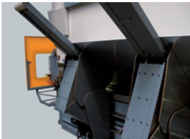
To support long and heavy or small and thin sheets during the bending process, the machine can be equipped with a hydraulic sheet following system. (photo: long arm version)
